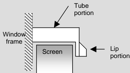
Removal: Turn each clip so its lip is facing away from the screen and is no longer holding the screen frame. Remove the screen.
