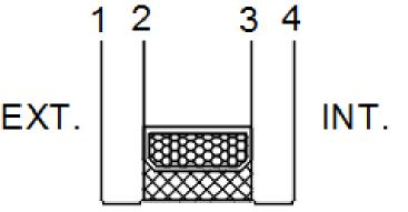
• Option for ceramic frit or opaci coat located on Surface #2 or #4. If ceramic frit or opaci coat is located on surface #2 then a Low E coating is not available for this application. Surface #4 is recommended.
