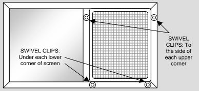
Removal: Turn each clip so its lip is facing away from the screen and is no longer holding the screen frame. Remove the screen.
