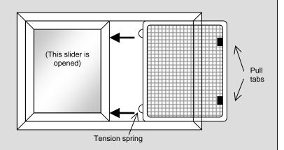
Removal: Compress the side with the tension springs and push (for 6000 series) or pull (for 8000 series) each pull tab. Remove the screen.
