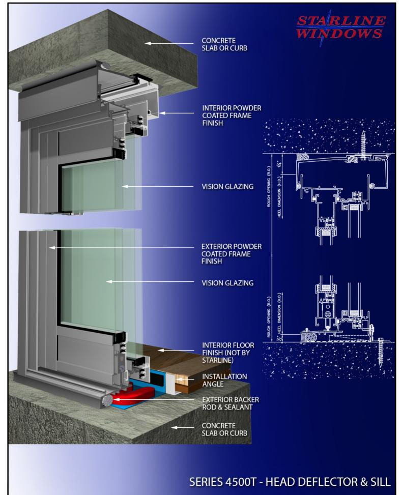
THIS DETAIL IS A SUGGESTED METHOD OF INSTALLATION AND DOES NOT REPRESENT A DETAIL THAT IS SUITABLE FOR A SPECIFIC PROJECT. TO CONFIRM PROJECT SPECIFIC DETAILS, PLEASE CHECK WITH YOUR WATERPROOFING/BUILDING ENVELOPE CONSULTANT.
