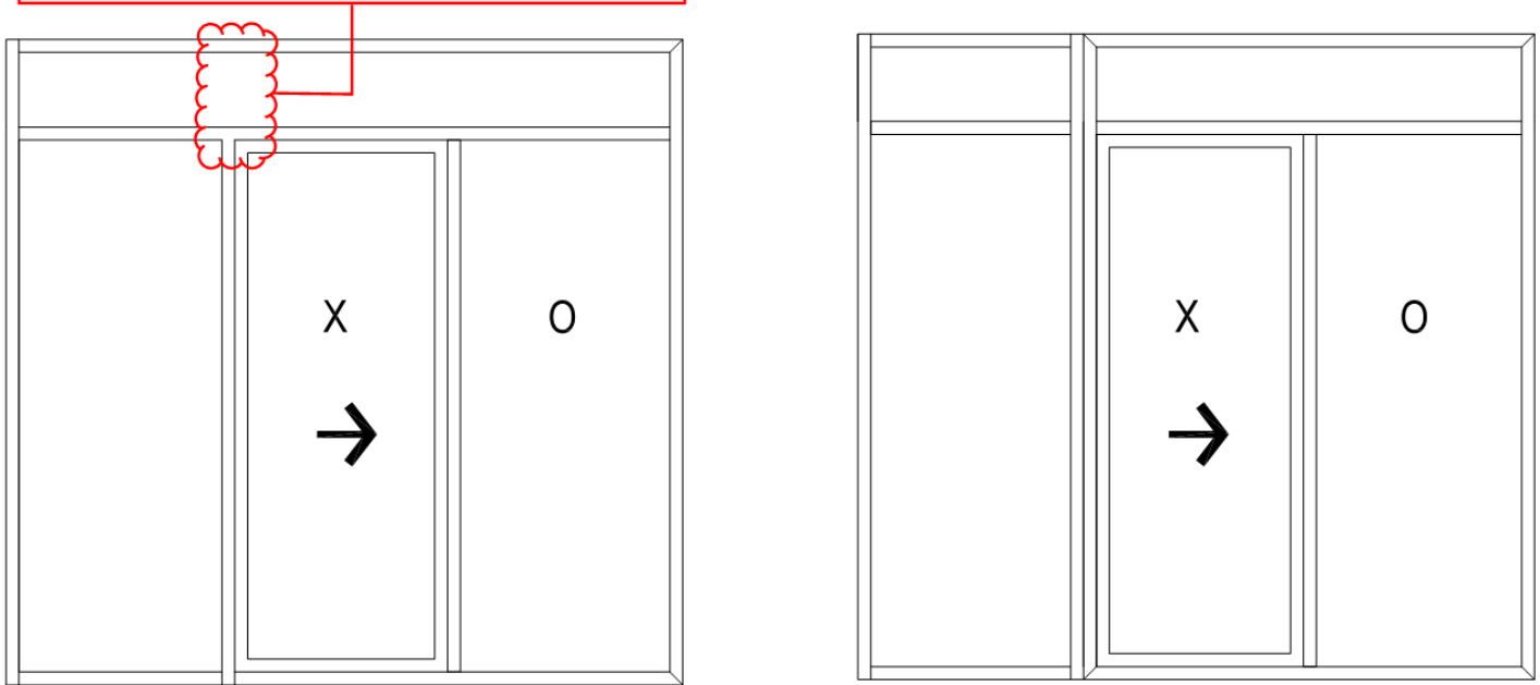
FIXED WINDOW COUPLED TO A SLIDING DOOR
