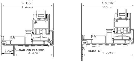
SHIMS ARE TO BE 2" WIDE HIGH IMPACT PLASTIC SHIM @ 4" O.C., TO PROVIDE 50% LEVEL SUPPORT OF WINDOW SILL. (OPTION TO BE SUPPLIED BY STARLINE)
